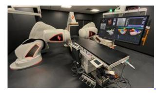
Procedure room equipped with Stereotaxis Robotic Magnetic Navigation (RMN) system for minimally invasive endovascular intervention. Robotic cardiac ablation is performed using a soft magnetic catheter navigated inside the heart by a physician seated at a computer cockpit. The physician navigates the catheter using precise, robotically actuated magnets positioned on either side of the patient.
