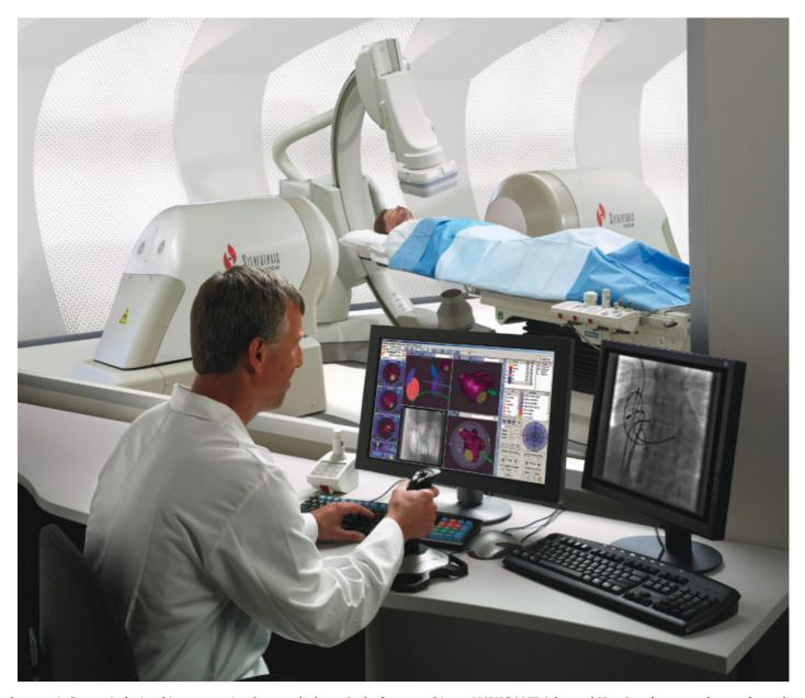
Our Stereotaxis System is depicted in a composite photograph above. In the foreground is our NAVIGANT Advanced User Interface control center located outside the cath lab, with a joystick used to navigate disposable interventional devices. Depicted in the adjacent cath lab shown in the background is our NIOBE cardiology magnet system, which utilizes two permanent magnets to govern the motion and orientation of the disposable interventional devices.
